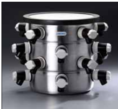
7522900 16-Port Drying Chamber 13.0" h x 13.0" diameter (33 cm x 33 cm), type 304 stainless steel, 3/4" thick acrylic lid with neoprene gasket, complete with 16 neoprene valves
